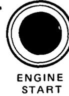
Press button to energize starter solenoid. The ENG TEMP light will come on while the button is depressed. Release button when engine starts.
