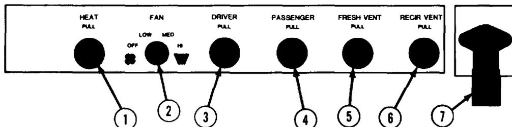
**Figure 2-5. Lower Control Panel.**
