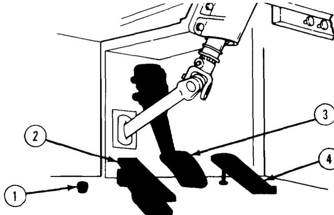
Figure 2-7. Cab Floor-mounted Foot Controls.
