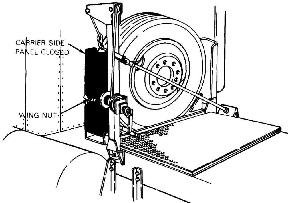
1. With the spare still mounted in the tire carrier, run the end of the cable through a wheel opening, wrap it around the tire and secure the snap back to the cable.
