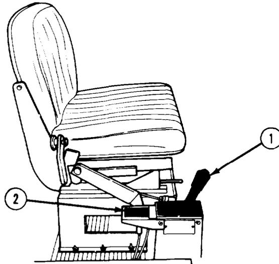
Figure 2-8. Transmission Range Selector Control and Sliding Fifth Wheel Control.
