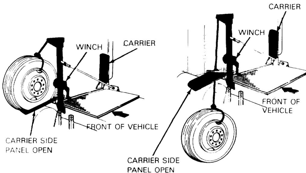
7. When the wheel and tire assembly is on the ground, detach the cable and leave it paved out in readiness for lifting the flat.
