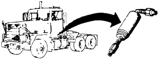
The diagram shows a side view of a truck. A curved arrow points from the driver's side door area to a detailed illustration of a fuel heater, which is a cylindrical component with a mounting bracket and a fuel inlet/outlet.
