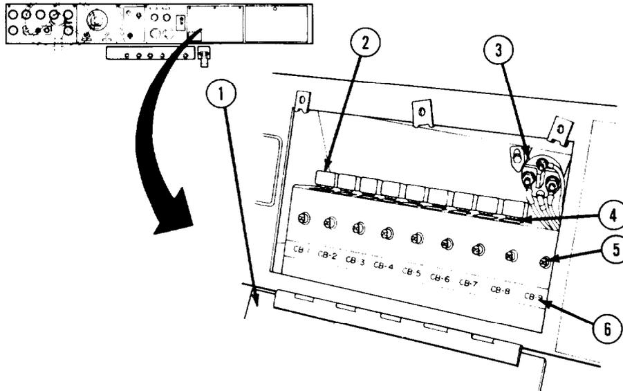
Figure 2-6. Circuit Breaker and Relay Access Panel.
