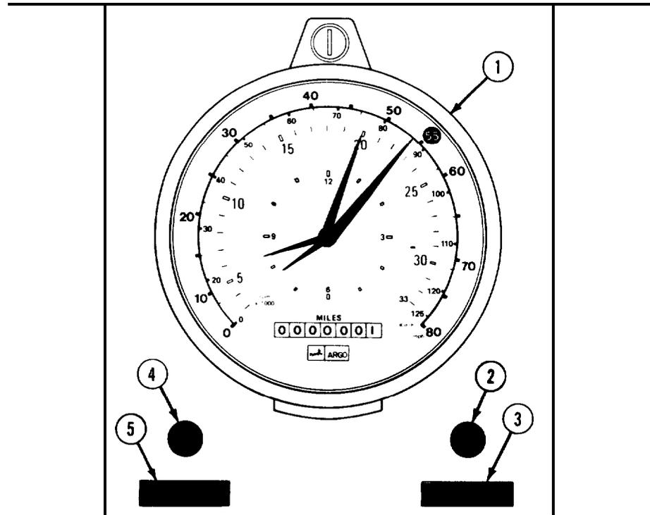
**Figure 2-3. Tachograph Section of Instrument Panel.**
