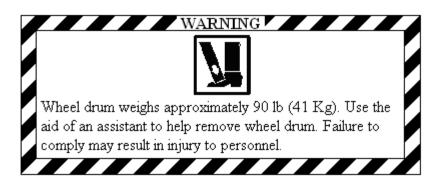
25. Install wheel drum (1) on wheel end hub (2).
